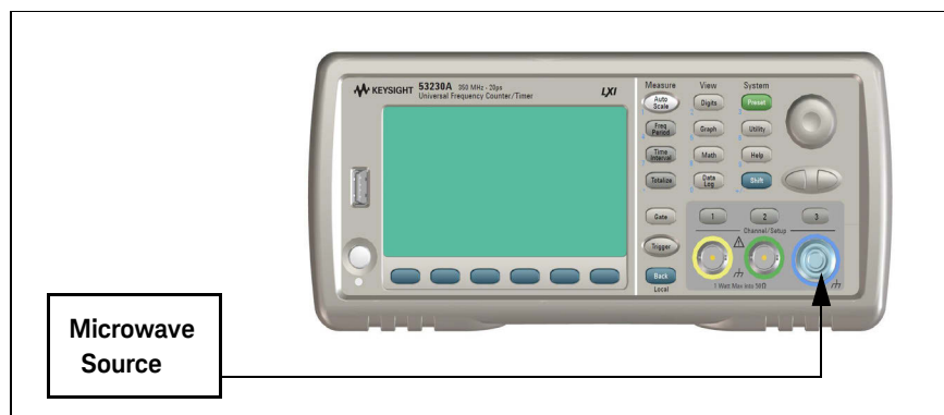
Figure 2-7 Microwave source connection to Channel 3
