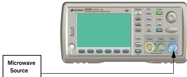
Figure 2-8 Microwave source connection to Channel 3
