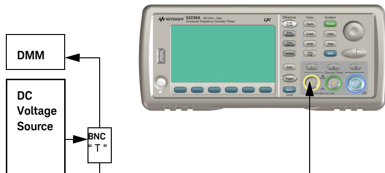
Figure 2-6 DC voltage source and DMM connections
