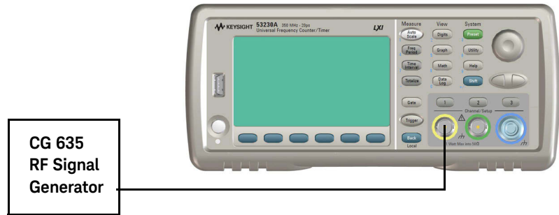
Figure 2-5 Oscillator calibration setup
