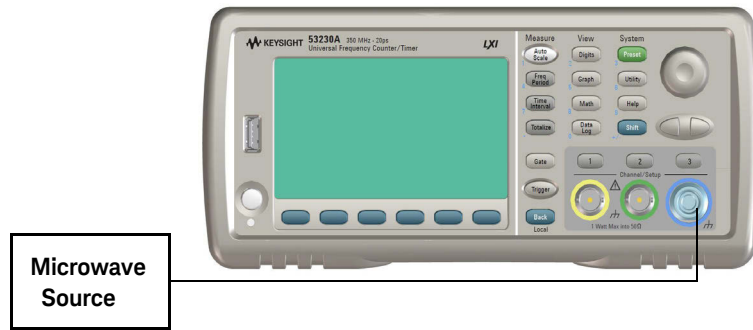
Figure 6-2 Microwave source connection to channel 3
