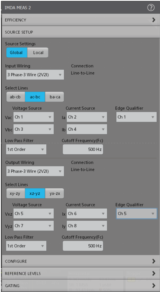
Configure wiring and filters to perform efficiency measurements for an Industrial motor
