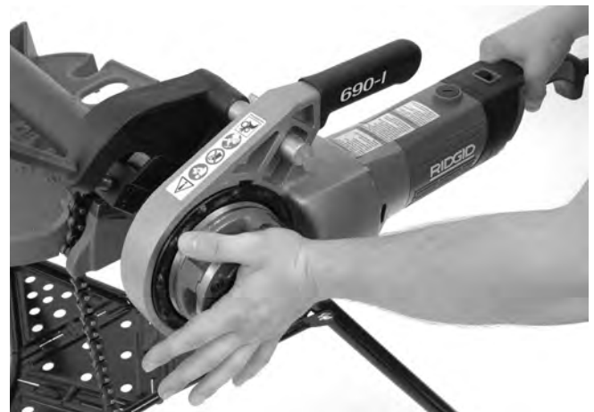
Figure 13 – Starting the Thread
