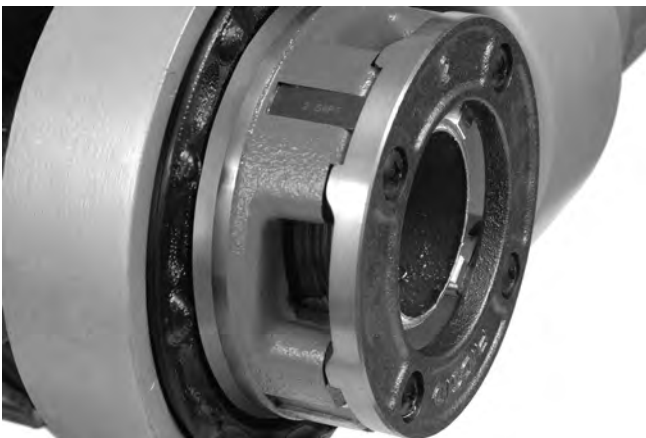
Figure 15 – Pipe Even with Edge of Dies
