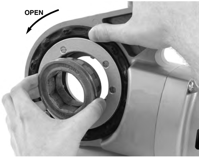
Figure 8 – Installing Adapter Into 690-I
