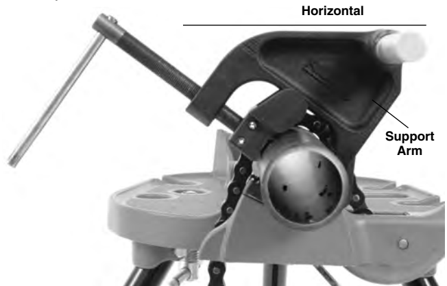
Figure 11A – Positioning the Support Arm
