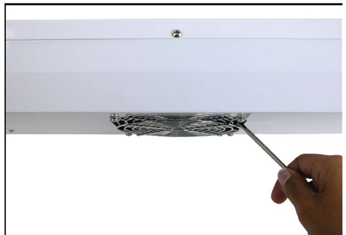
Figure 10. Shorting the ionizer's two fan grills
