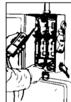
With power on: Place tester across the "source" side of one fuse and the load side of an adjoining fuse. If no or low voltage is indicated, the fuse next to the load side prod is blown. If line voltage is indicated, the fuse next to the load side prod is OK. Repeat the same test with the prods on the opposite side of the same two fuses to check the other fuse.
