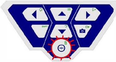
Fig. 23 Control panel of Wöhler VIS 250 / 350 - ON/OFF key framed by flashing light
