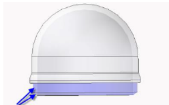
Fig. 34: Fitting the camera dome
