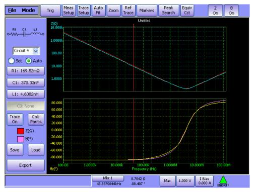
This example shows the measurement traces for a film capacitor and the close fit of the calculated traces using Circuit 4.
