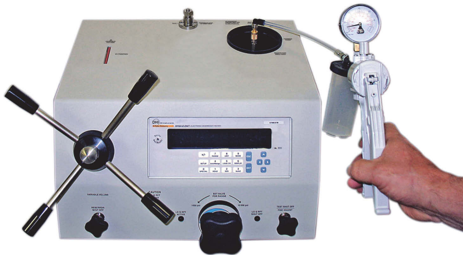
Figure 3: Evacuating the E-DWT-H with fill kit
