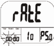
Fig. 19: Setting the sampling rate (hours)
