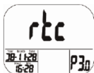
Fig. 13: Setting clock and calendar (rtc: real time clock)
