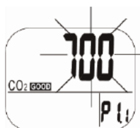
Fig. 8: Setting the upper limit of the good level.
