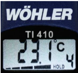
Fig. 5: Bar indication Hold function
