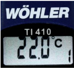
Fig. 2: Temperature indication sensitivity step 1
