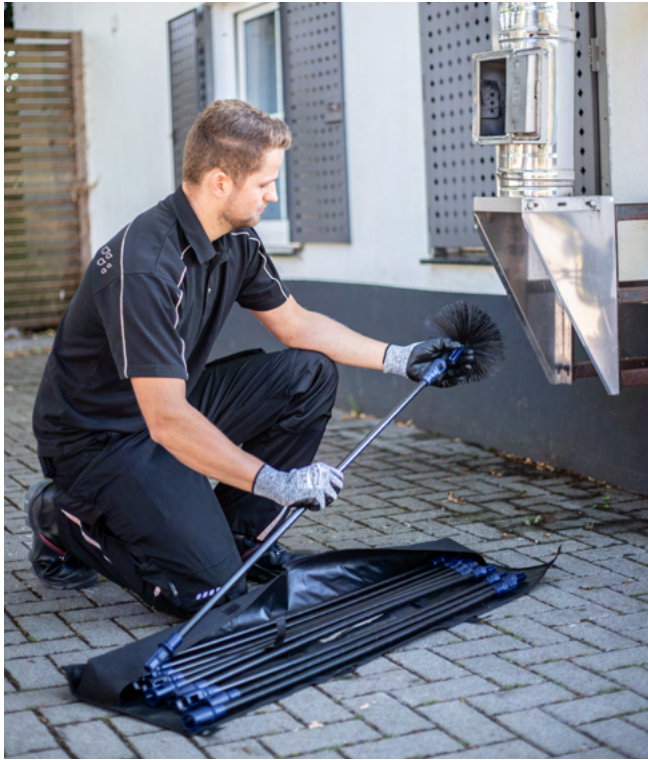
Unused tools can be placed on the open carrying bag to keep the working area clean.
