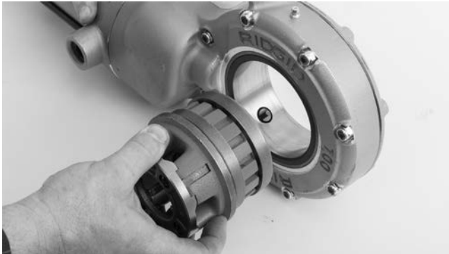
Figure 4 – Installing Die Heads into 700 Power Drive
