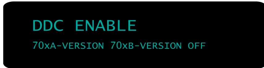
Figure 26: Front panel DDC enable menu
