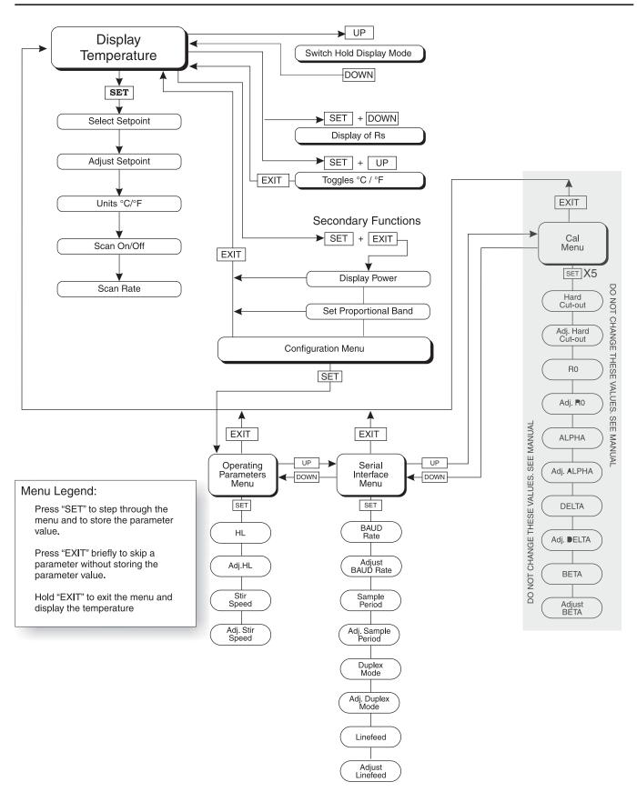
Figure 7 Controller Operation Flowchart
