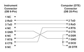
Figure 8 Serial Cable Wiring
