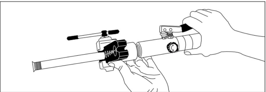
4.) Assemble the hydraulic pump. Turn the hydraulic bar until it is tight. Close the relief valve knob and pump handle until it becomes firm.
