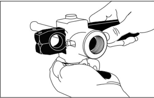
3.) Slide the yoke over the bar until the bars line up to the copper tube at the selected size. Tighten the handle on the yoke.
