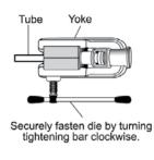
4) Grasp the yoke and rotate the hydraulic cylinder clockwise until it stops. (The adapter should engage the die.)
