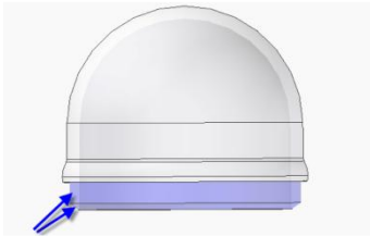
Fig. 22: Fitting the camera dome
