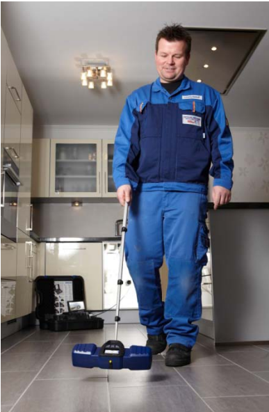
Fig. 11: Localizing the camera head underground
