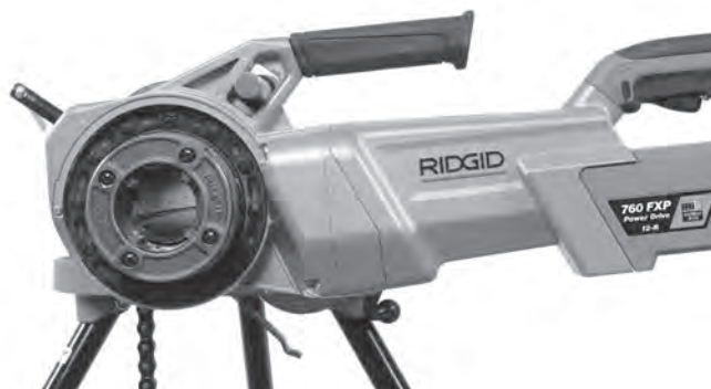
Figure 11 – Orientation appropriée du 760 FXP Power Drive
