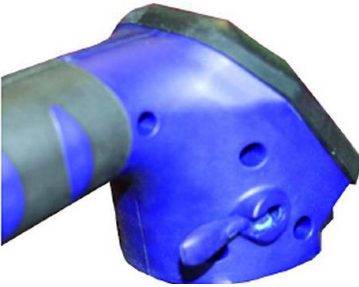
Fig. 16: vertical position of the lever - transport lock activated
