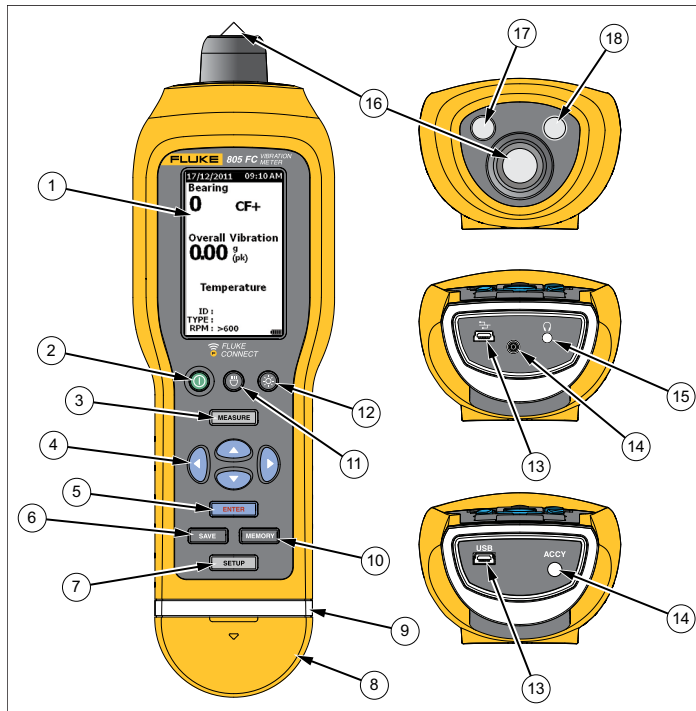
Figure 1. Meter Controls and Connections
