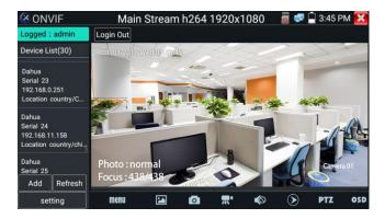
Click the button "Refresh", the tester will scan the ONVIF camera again. Click the newly displayed ONVIF camera on the "Device List". The tester will show the IP camera's relative information and settings.
