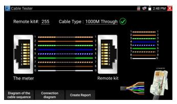
Test LAN cable or telephone cable.
