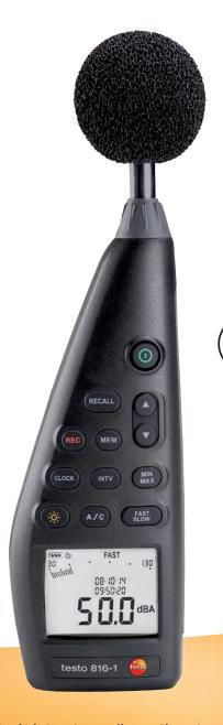
The testo 816-1 is ideal for sound level measurements at workplaces, in commercial, and public areas. With the touch of a button, the 816-1 can be switched from Slow (1 sec.) to Fast (125 ms). It is also possible to switch between the frequency weighting characteristic curves A and C. Characteristic curve A corresponds to the sound pressure sensitivity of the human ear, while characteristic curve C can evaluate low-frequency components of a noise.
