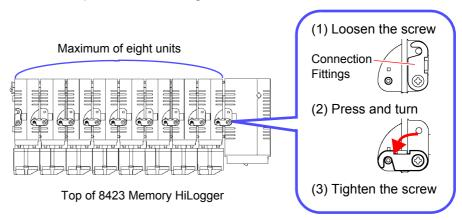
3. Attach the supplied connector cover to the unit on the very left side when looking from the front.
