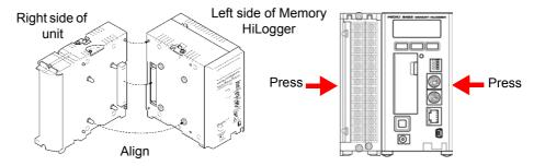
2. Secure the unit in place with the connection fittings at the top and bottom of the unit.
