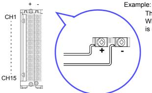
The 8948 Voltage/Temp Unit When a thermocouple cable is connected
