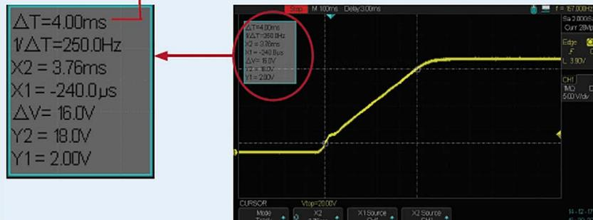
The 8500B Series can measure the rise or fall time from a specified start and stop voltage level of the measured input without the need for an oscilloscope. This function can also be used as an internal timer to count how long the input has been enabled.
