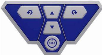
Fig. 8: Control Panel Wöhler VIS 300
