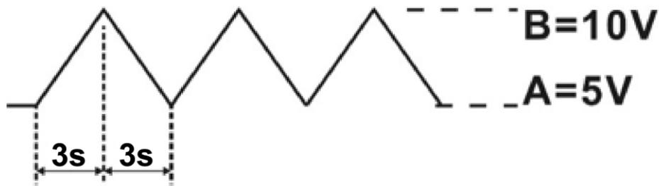
Figure 14 - Transient Mode: Example 3
