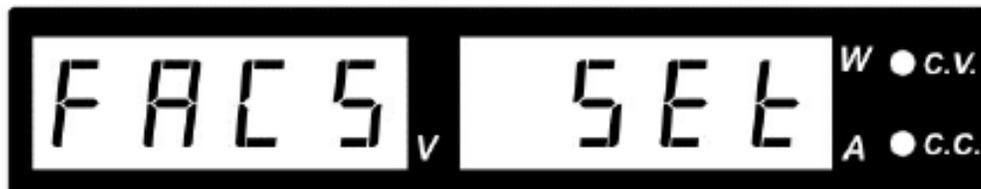
Figure 5 - Factory Reset Display
