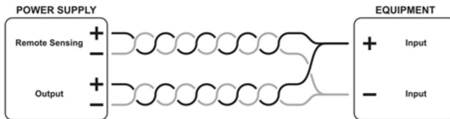
Figure 22 - Remote Sensing
