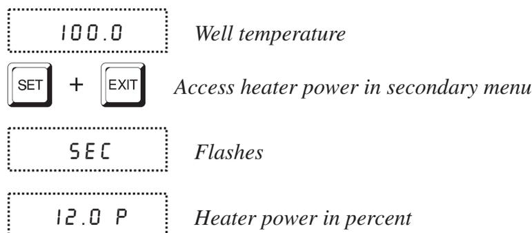
To exit out of the secondary menu press and hold “EXIT”. To continue on to the proportional band setting function press “EXIT” momentarily or “SET”.
