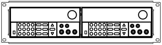
To rack mount two instruments (models 9120A, 9121A, 9122A, 9123A, 9124 only) side-by-side, order rack mount kit IT-E151, In this case you don't need to use the front cover panel.
