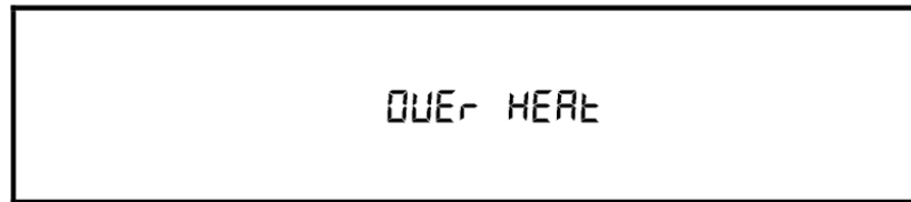
Figure 16 - Over Temperature Protection Warning
