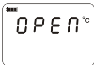
Figure 6: Display when no probe is detected
