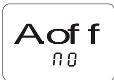
Figure 9: Disabling the auto off function
