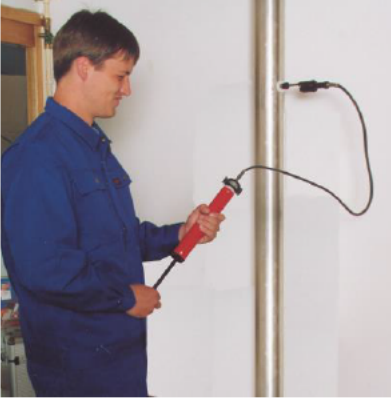
Fig. 4: Extracting the smoke gas
