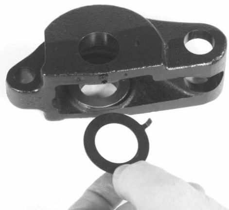
**Figure 18 – Inserting Tabbed Thrust Washer**
