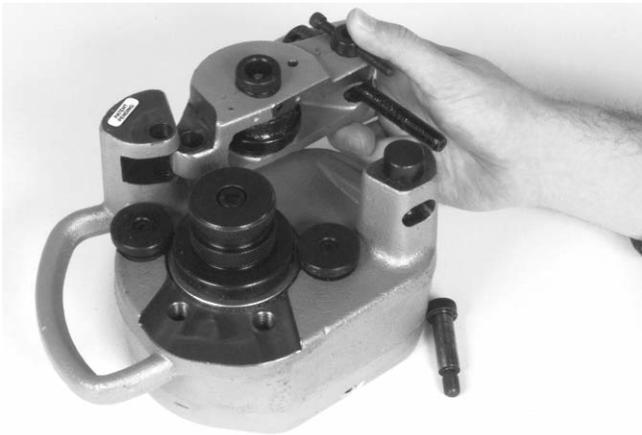
**Figure 15 – Removing Feedscrew**
