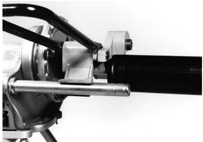
Figure 6 - Square Pipe & Pipe Support
