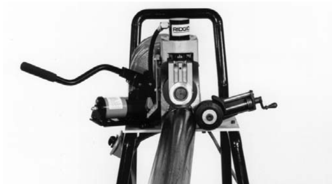
Figure 7 – Offset Pipe on 918-I (exaggerated for clarity)
