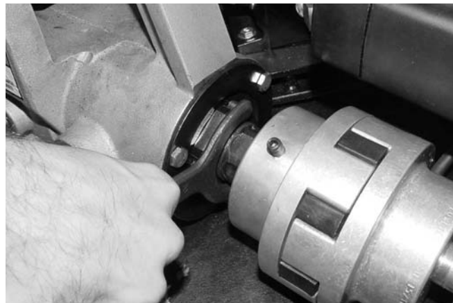
Figure 14 – Loosen and Remove Drive Shaft Retaining Nut
