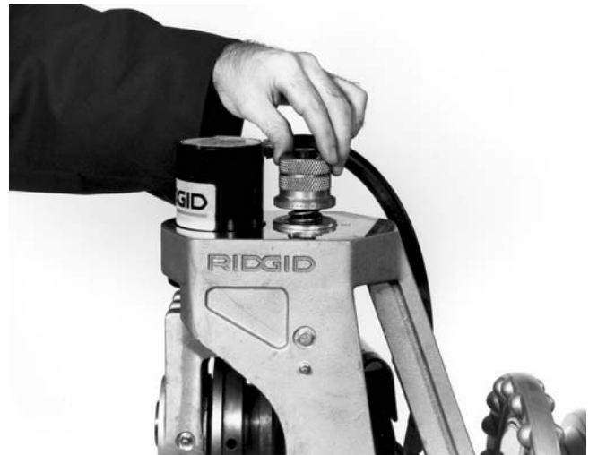
Figure 8 – Close-up of Depth Adjustment Knob Being Turned Down Against Top Casting
