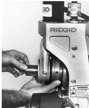
Figure 12 – Remove Groove Roll Shaft and Groove Roll
