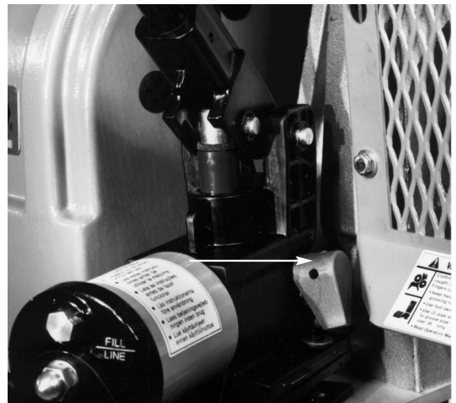
Figure 4 – Close-up of Release Lever on 918-I Pump
