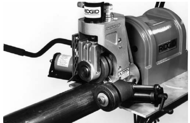
Figure 10 – Adjusting Pipe Stabilizer
