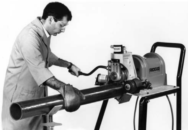
Figure 9 – Grooving Pipe While Exerting Light Hand Pressure Toward Operator
