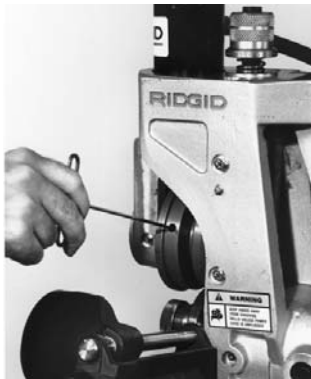
Figure 11 – Loosen Set Screw in Groove Roll
