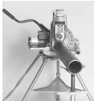
Figure 12 – Offset Pipe on 918 in FORWARD Position
