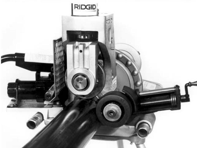
**Figure 23 – Stabilizer Positioning**
