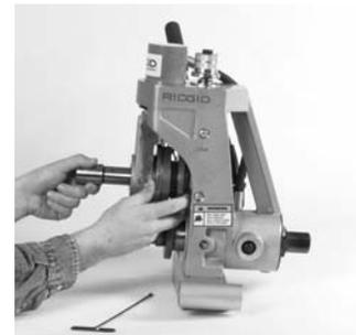
**Figure 18 – Removing Retaining Shaft and Groove Roll**
