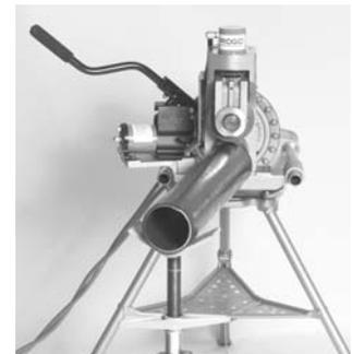
Figure 13 – Offset Pipe on 918 in REVERSE Position
