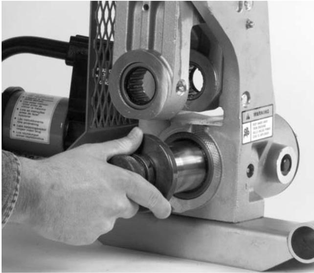
**Figure 20 – Removing Drive Shaft**
