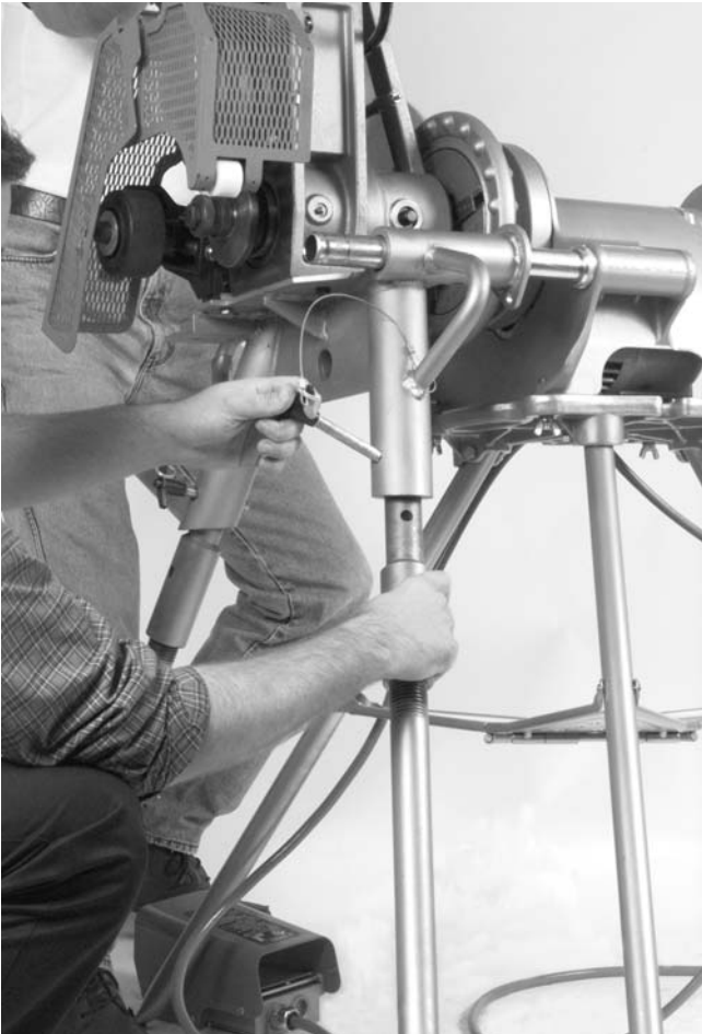
Figure 5 – Installing Legs Into the Groover Base
