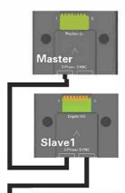
The TL983P adapters connect to the Digital I/O connector on the rear of the AC source. Standard RJ45 communication cables connect each adapter to route the 3-phase synchronization signal from the master to the slave units.
