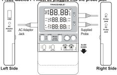
labeled "P1" and probe labeled P2 must be plugged into the probe jack labeled "P2".
