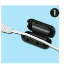
Lay the cable along the center of the suppressor with the connector to your left.
