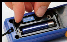
Attach to enable Bluetooth® wireless technology
