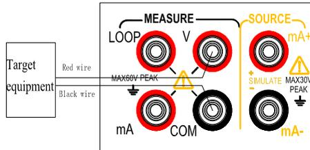
Step 1: Ensure that the measurement lead is disconnected from the equipment under test.
