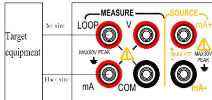
Step 1: Ensure that the measurement lead is disconnected from the equipment under test.
