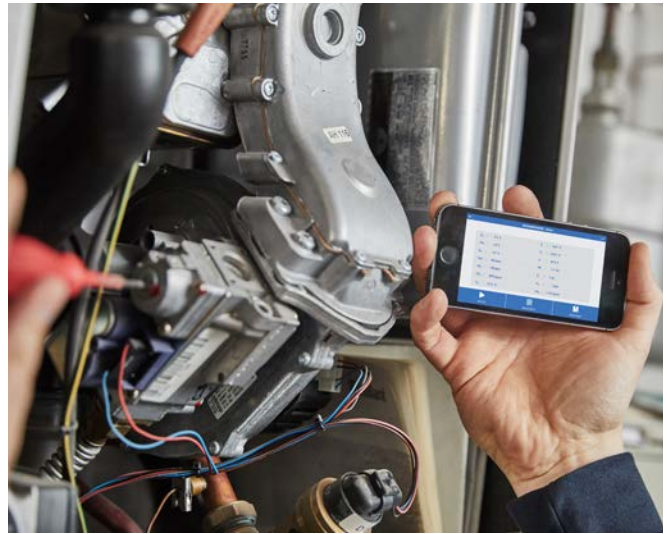
Wöhler A 450 app: Displaying the measured data on a mobile device.
