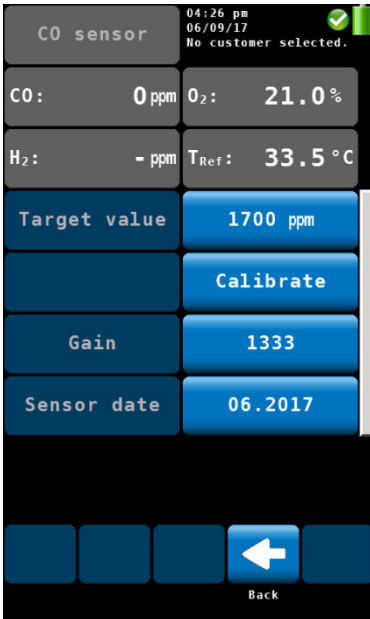
Fig. 56: Entering the calibration values in the calibration menu (only CO-sensor)
