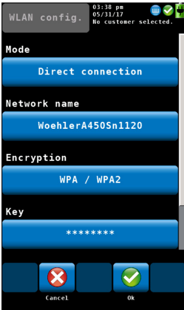
Fig. 35: WLAN configuration – Direct connection
