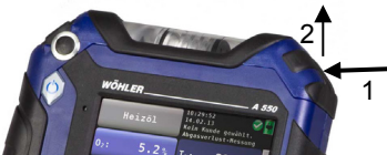
Fig. 65: Open the condensate trap compartment
