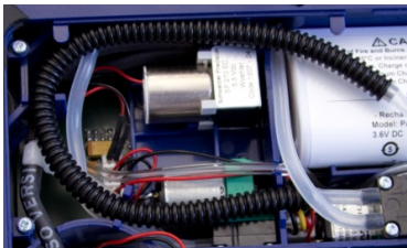
Fig. 75: Corrugated tube, correctly positioned
