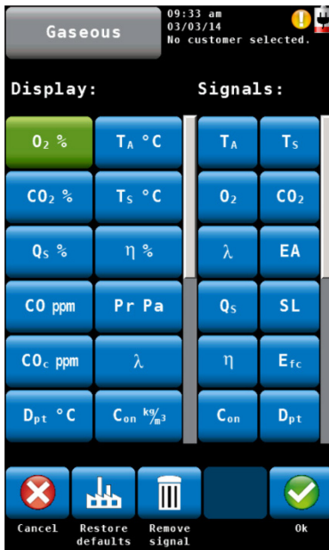
Fig. 58: Configuration of the readings segment.
