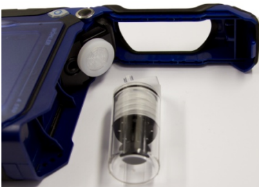
Fig. 65: Open the condensate trap compartment
