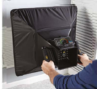
Included expansion hood captures airflow from grilles up to 24" x 24" (.6 x .6 m)
