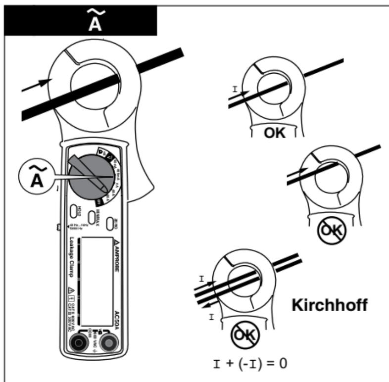
For incorrect measurement, the display equals zero. In compliance with Kirchhoff's current law, the sum of all currents equals zero. However, this measurement layout in conjunction with a very sensitive current clamp can be used to measure leakage currents.
