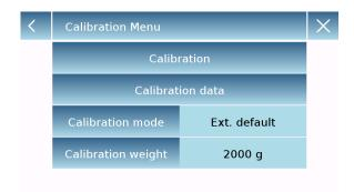
In the calibration menu, you can calibrate, display and print the data for the last calibration and set the calibration mode.
