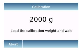
Load the required calibration weight or tap the "**Abort**" button to cancel the calibration procedure.
