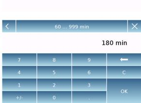
To change the auto-calibration range, tap the "Calibration Range" key and set the desired range between 60 and 999 minutes.
