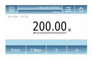
If you work with weighing boxes, first zero the balance. Place the container and press the "-T-"key.
