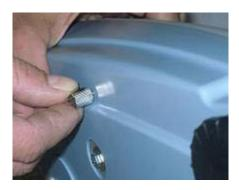
**Level** the balance by adjusting the legs on the front of the balance. Some models also have an adjustable leg on the rear left.
