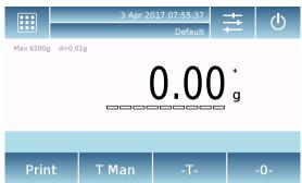
In the weighing screen, the area displaying the weight shows the value of the weight on the weighting plate.
