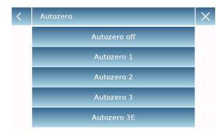
Autozero: automatic correction zero constantly adjusts the zero value. These variations may be due, for example, to dirt that can be deposited on the plate. You can disable this function by selecting "Off" mode. Level 1 is the one with minor correction until it reaches level 3E which is the maximum correction
