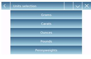
On the "Units Selection" screen, all available weighing units are immediately displayed. Tap the desired unit to select it and enable it.
