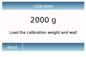
Load the required calibration weight or tap the "**Abort**" button to cancel the calibration procedure.
