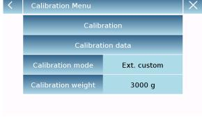
After selecting the "mode of choice", tap the Weight Setting button to set the desired weight value.
