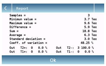
After tapping the "End" key, the screen with the result of the weighing statistics is displayed.
