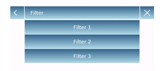
Filter: the filter function allows to speed or slow down the balance response according to weighing requirements and environmental conditions. By selecting Level1, the response will be immediate, but the balance will remain more sensitive to environmental disturbances such as ventilation and vibration. By increasing the level, the response will be slower and the indication more stable.
