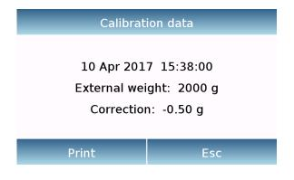
Calibration date: in the calibration data screen, you can check the date when the last calibration was performed, the mode with which it was performed, the weight value used, and the correction made with respect to the previous calibration. By tapping the "Print" button, you can print the displayed data.
