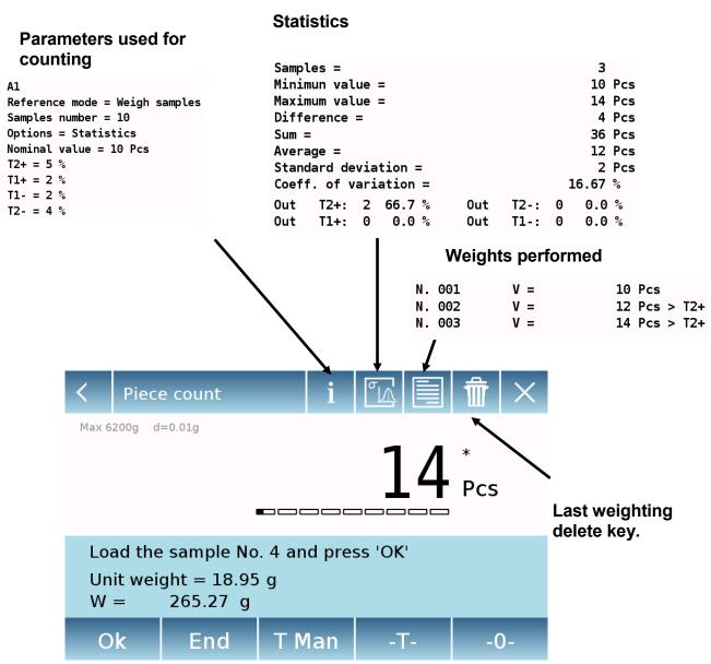
Tap the "Ok" key to capture a new weight and tap the "End" key to end the capture and perform the final statistical calculation.
