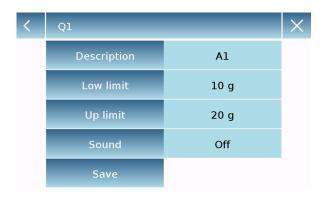
To activate the function, enter the values for the "lower limit" or "upper limit" or both, according to the method you want.
