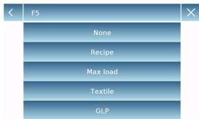
То remove function, press the key corresponding to the function you want to remove and select "None" in the list.
