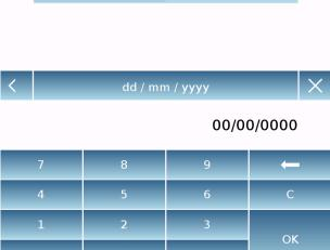
A numeric keypad will be displayed for entering the date and time in ""dd/mm/yyyy" mode for the date and "hh:mm:ss" for the time
