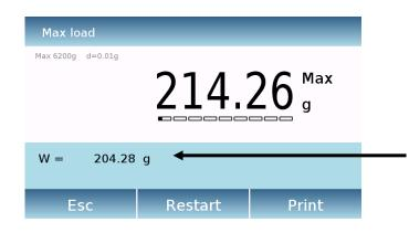
Once the tested sample breakage load is reached, the maximum weight will be displayed.
