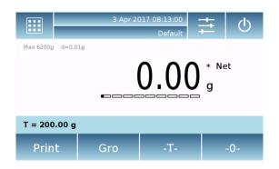
The **Net** symbol on the display indicates the net weight. Press "**Net**" to see the gross weight "**Lrd**".
