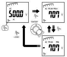
2. In AC A mode, select "♠" indicator then press the navigator key for more than 2 seconds to enter PEAK HOLD mode. To exit PEAK HOLD mode, just press the navigator key for more than 2 seconds to return to the "♣" indicator.
