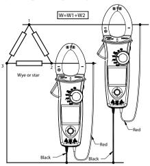
B. 3 phase 4 wire balanced / unbalanced Step1. Set the rotary switch to the "W" position Step2. Using the Navigator key to choose the "W" mode.
