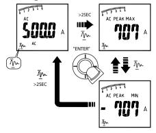
In PEAK HOLD mode, the meter is activated to save the positive peak value and negative peak value. Positive peak value is displayed in PEAK MAX mode. Negative peak value is displayed in PEAK MIN mode.
