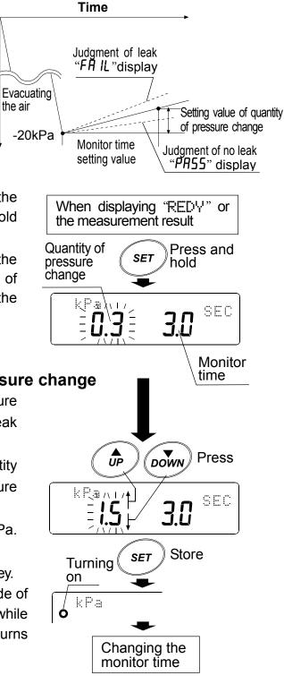
\* If the quantity value of pressure change is insufficient when measuring, *"FR IL"* may be displayed by changing the measurement system pressure (Leak Tester, adapter, attachment).
