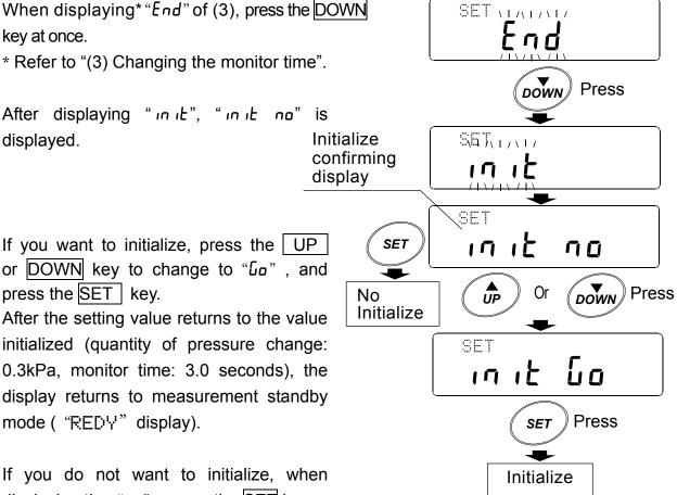
If you do not want to initialize, when displaying the "no", press the SET key. The display returns to measurement standby mode ( "REDY" display) after displaying "End".
