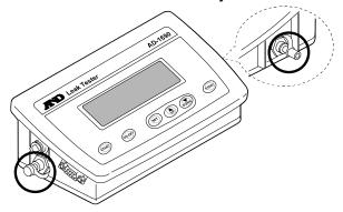
Confirm that the filter unit is installed in the holder located on the main unit bottom side correctly.
