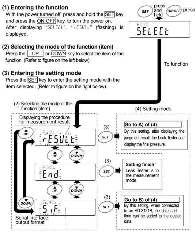
\* Press the SET key while "End" is flashing.
