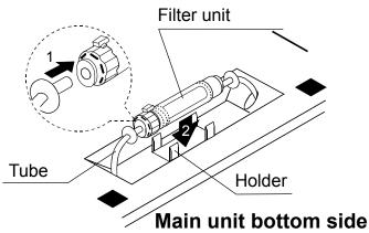
\* If particles of dust invade the tube, they may cause trouble. When replacing the filter, be careful that no dust invades the instrument.
